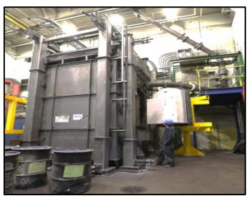
New 1-tonne capacity Energy Recovery Coke Oven
